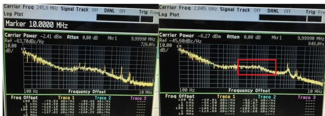
Figure 5. PLL Reference Clock Phase Noise (Left), and Normal DAC Output Phase Noise at 2605 MHz at 5-MHz PLL Loop Bandwidth (Right)
