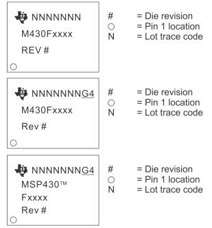
NOTE: Package marking with "TM" applies only to devices released after 2011.
