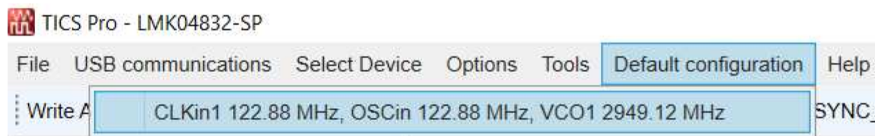
Figure 3. Selecting a Default Mode for the LMK04832-SP Device
