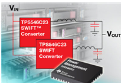
Figure 2. Stacking Two DC/DC Converters for Higher Load Currents.
