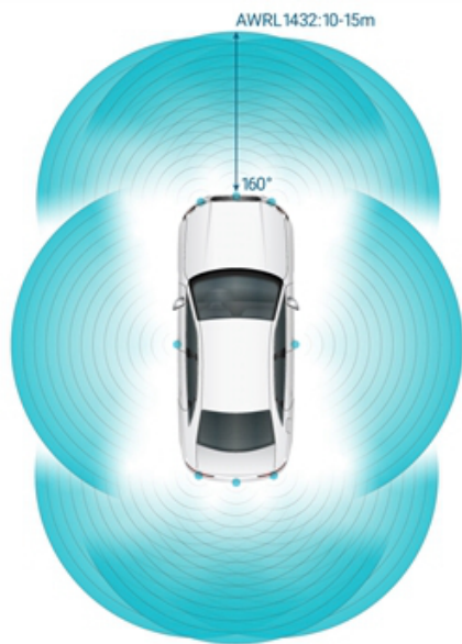
Figure 2. 360-degree coverage for park assistance using radar sensors
